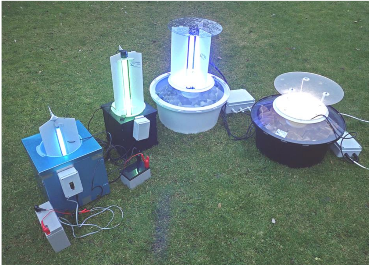
Examples of different types of moth trap (left to right): 6w actinic and 15w actinic both battery-powered, twin-30w actinic and 125w mercury vapour both mains-powered. The very bright 125w bulb was still warming up when this photo was taken and wouldn’t be recommended for gardens overlooked by neighbours! All are effective at catching moths.
